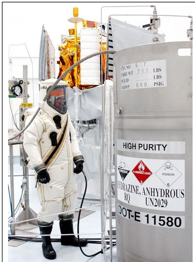
Figure 3.5-1. Hydrazine being loaded onto NASA's Messenger space probe
