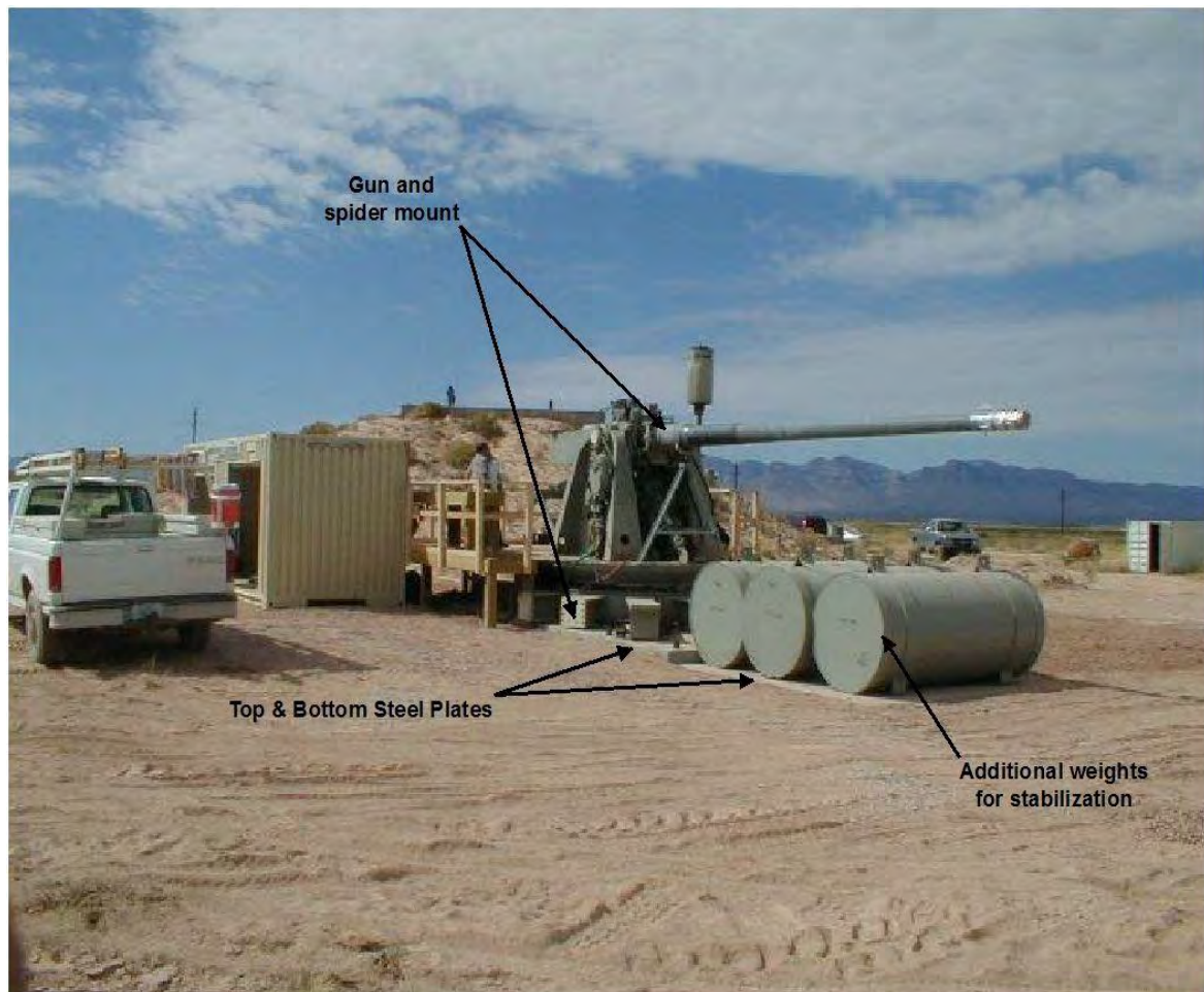
Figure 2-9: Powder Gun Installation at the White Sands Missile Range
