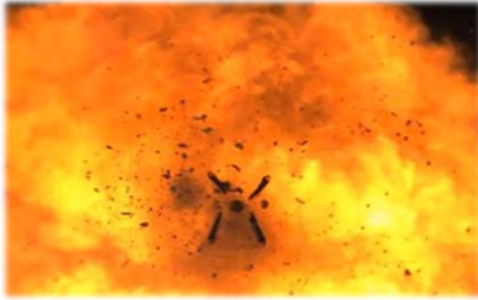
Figure 2-3: Sabot petals flying off the projectile after the projectile is launched. A single petal is depicted on the right.
