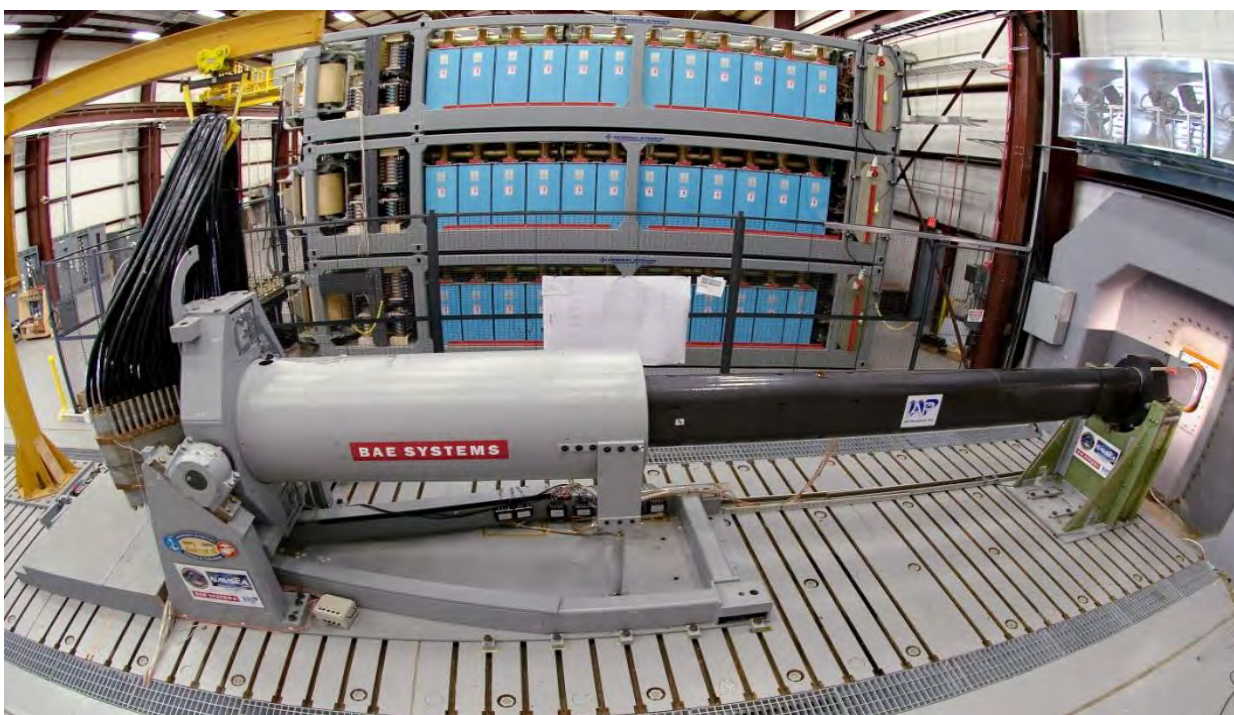
Figure 1-5: 32-megajoule prototype railgun in the Electromagnetic Launch Facility in 2012. The pulsed power system, composed of banks of electrical capacitors, is behind the gun.
