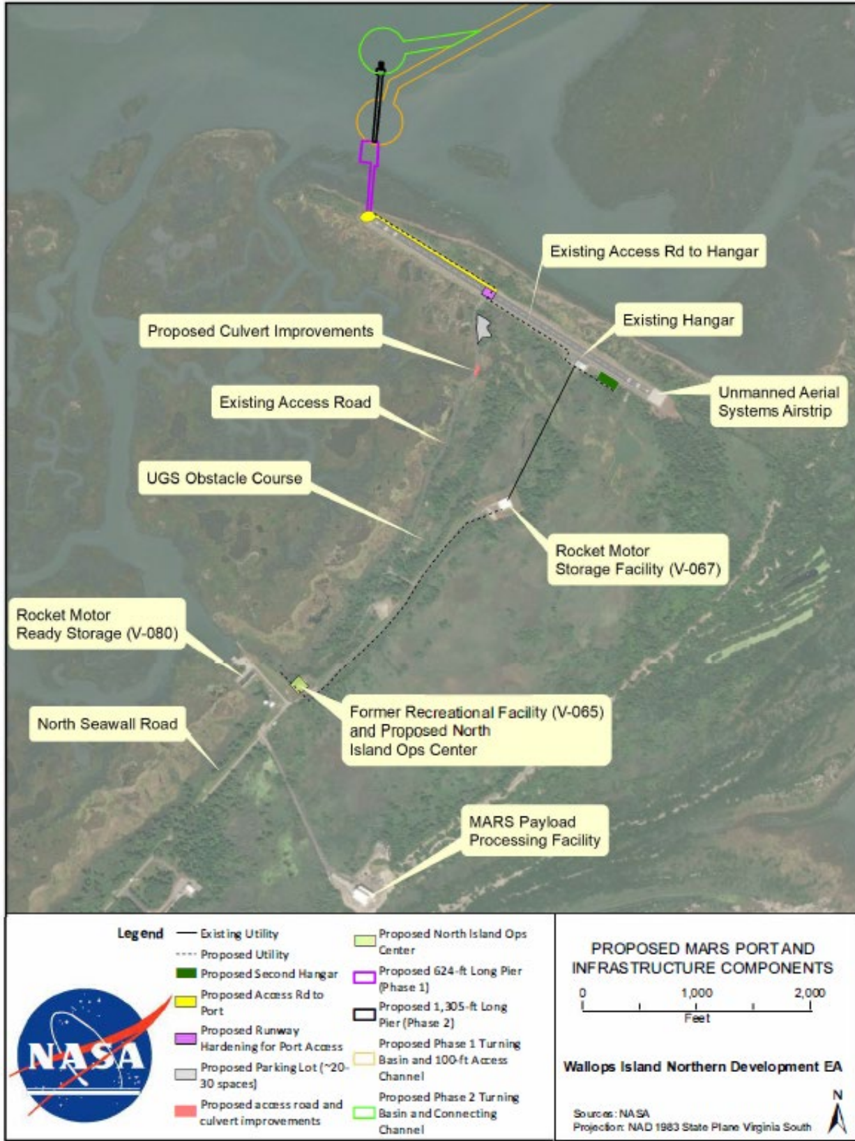
Figure 2: Proposed MARS Port and Infrastructure Components
