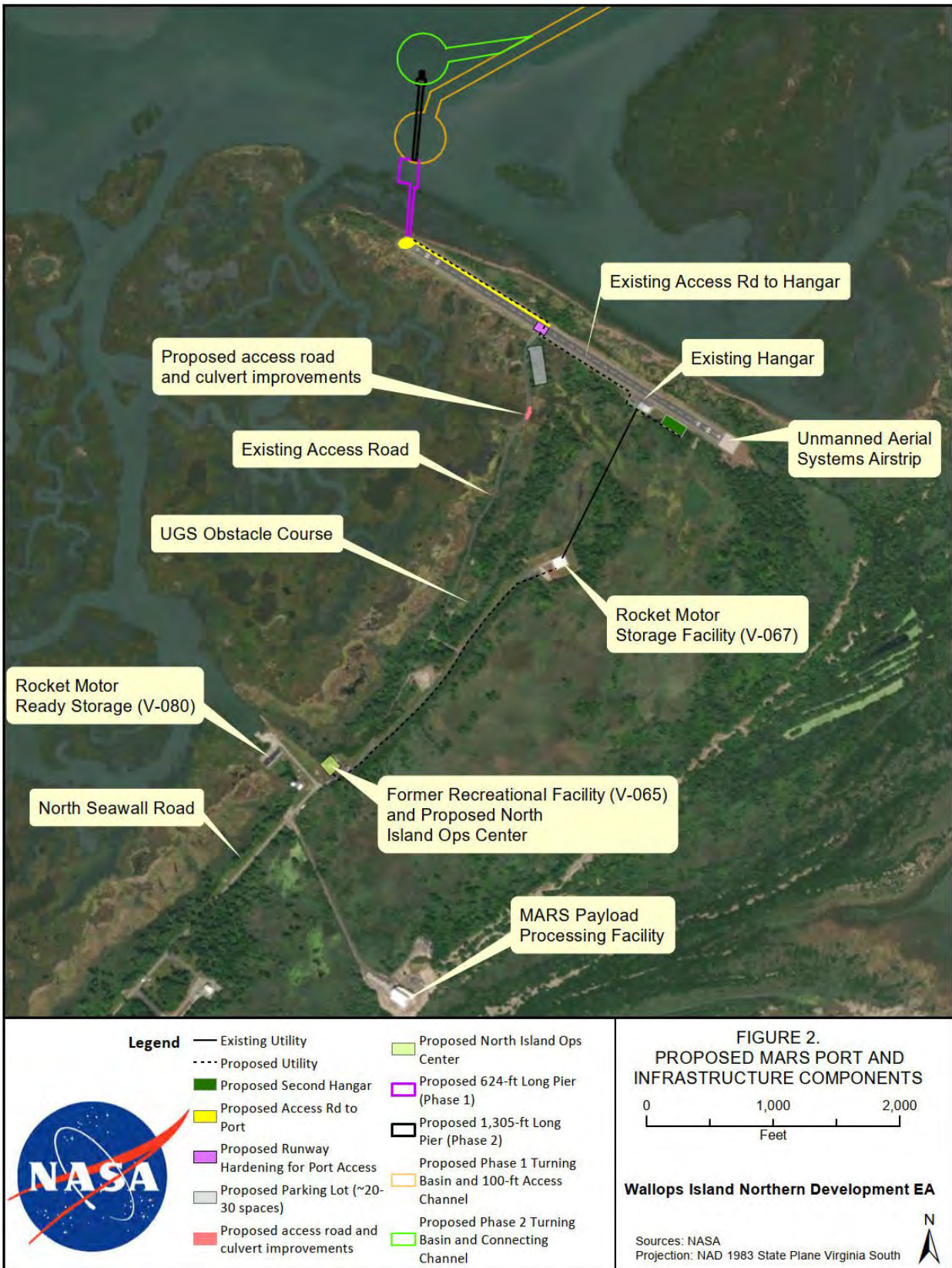
Figure 2. Proposed Mars Port and Infrastructure Components
