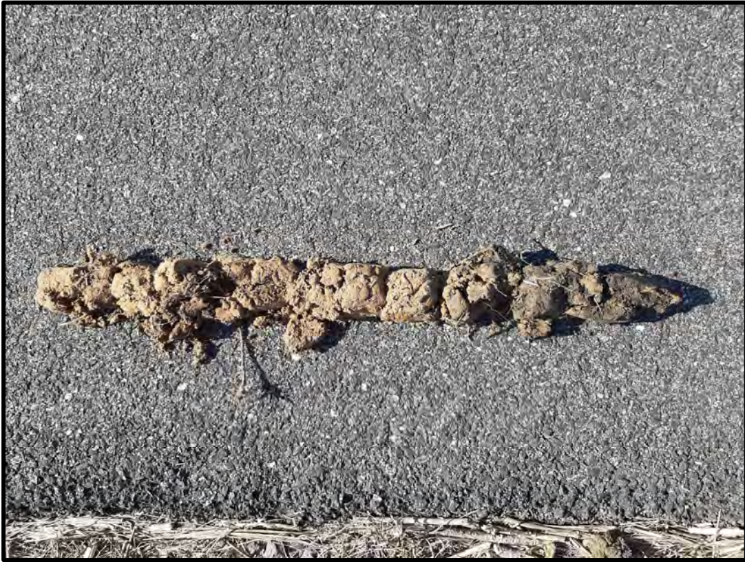
Photograph 11: Soil profile of upland roadway shoulder exhibiting sandy fill materials
