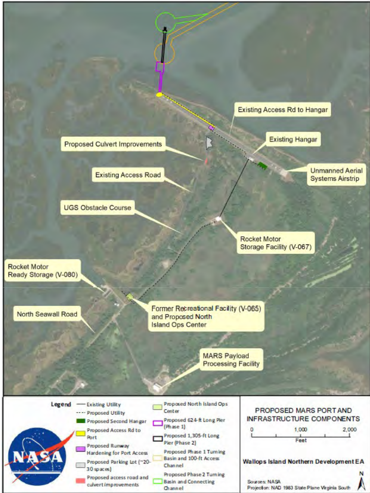
Figure 2. Proposed MARS Port and Infrastructure Components
