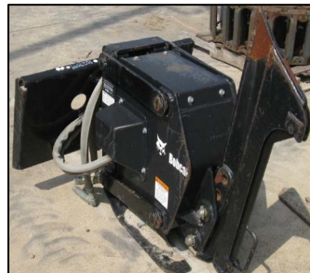
Photo 2-3. Vibratory plow attachment.
