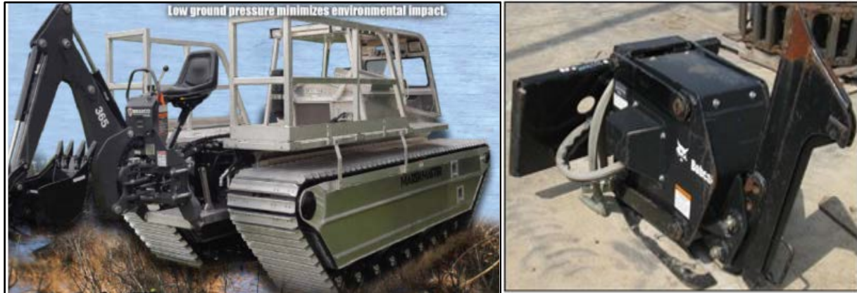
Figure 6. Example of Marsh Buggy and Plow Attachment
