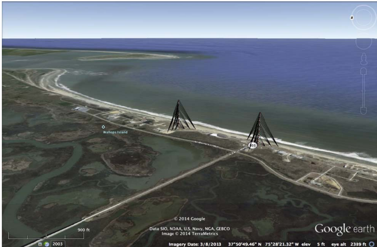
Figure 2. Three-dimensional rendering of potential tower sites. Guy wires depicted are worst-case and would likely be fewer per tower leg.
