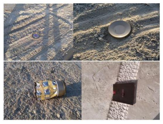
Figure 3-6: Mortar Lid, Sabot, and Forward Heat Shield Door Impacts
