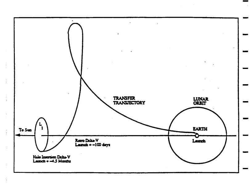
FIGURE 2 ACE TRANSFER TRAJECTORY AND HALO ORBIT
