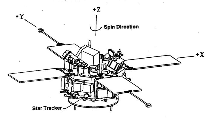
FIGURE 4 ACE SPACECRAFT DEPLOYED CONFIGURATION
