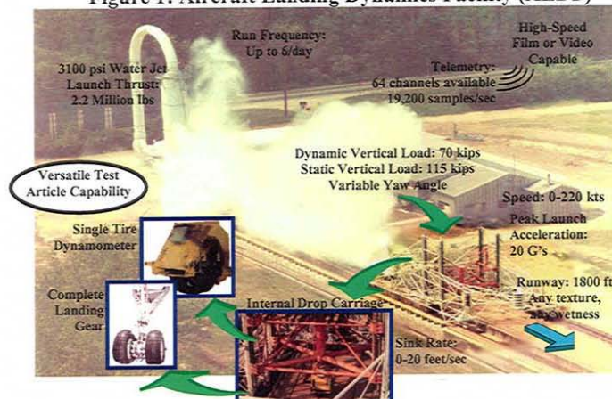
Figure 1: Aircraft Landing Dynamics Facility (ALDF)
