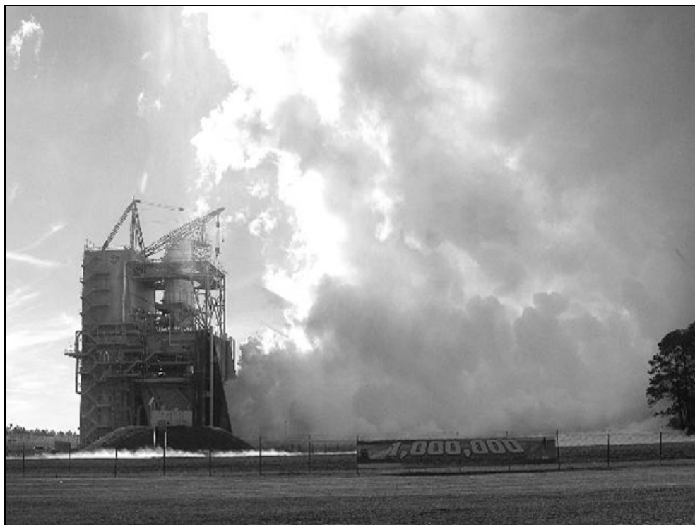
Figure 4-6. Testing of a LOX/LH Fueled Rocket Engine at SSC
